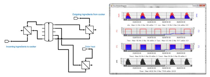
Figure 16: SOCO: flowsheet of the system simulation for combined heat integration and solar heat (left). Example of heat exchanger performance data visualization for the heat exchanger loading the heat storage with solar heat (right).
