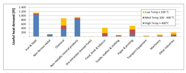
Figure 3: Breakdown of useful heat demand for EU-27 industry for 3 temperature levels for the main industry sectors in Europe.
