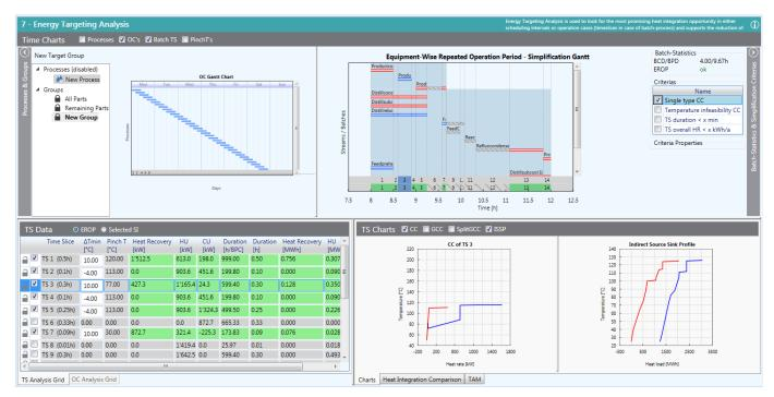
Figure 15: PinCH: screenshot of the Energy Target Analysis interface for simplifying repeated batch processes to most energy relevant time slices for direct heat recovery.
