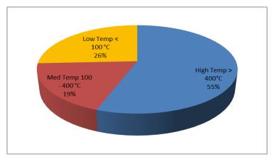
Figure 2: Breakdown of useful heat demand for EU-27 industry in 3 temperature levels.
