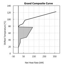
Figure 10: Heat pump matched against GCC (left), CCs after heat pump streams integration, but not yet deciding evaporator and condenser heat transfer matches (center), and GCC after taking out actual evaporator and condenser heat transfer matches (right) – Scenario 1 involving a 276 kW compression heat pump.
