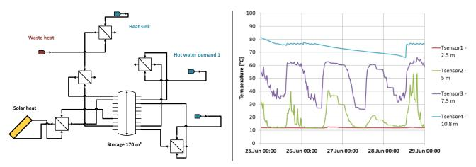
Figure 13: Flowsheet in SOCO which can be simulated to evaluate the performance of heat exchangers and storages (on the right) over time; combinations of solar heat and heat recovery can be analyzed.
