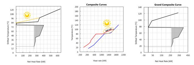
Figure 11: Solar heat integration (340 kW) matched against GCC (left), CCs after 340 kW solar heat integration (center), and GCC after taking out 300 kW solar heat supply actually matched with lye bath (right) – Scenario 3 solar heat supply.
